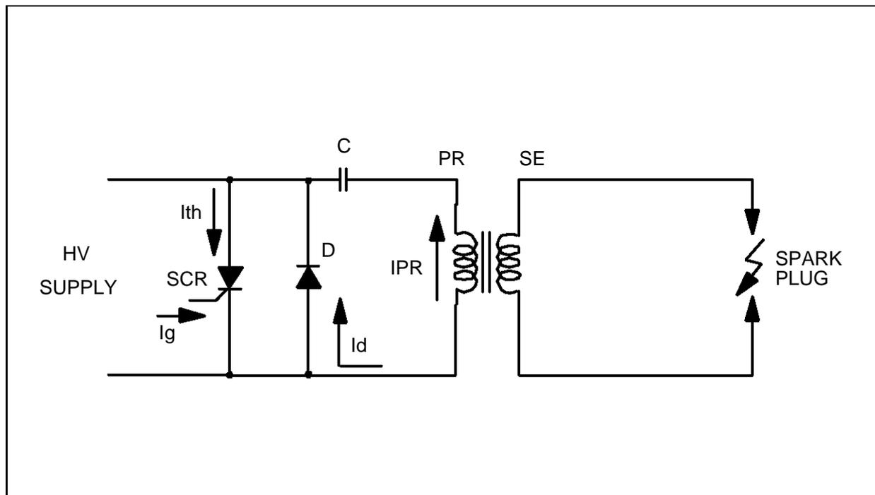
When spark is needed a current  $I_g$  is injected to the SCR gate which then fires the SCR. The SCR firing initiates the capacitor discharge which generates an alternative current.
