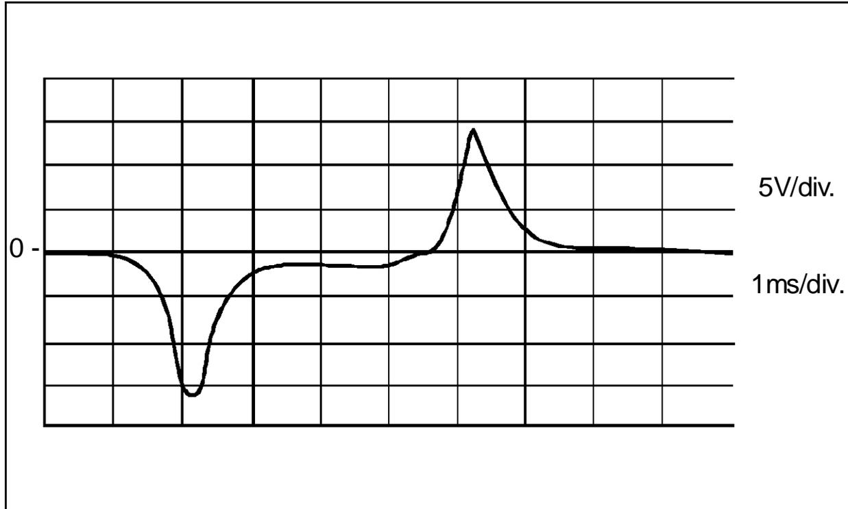
The sensor coil generates, at each engine revolution a signal as shown in figure 7.
