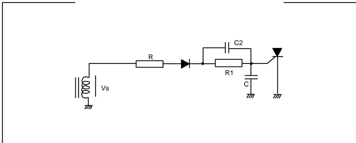
This gate drive circuit, using  $R1$  between 1 and  $10k\Omega$  and  $C1$  between 1 and  $10\mu F$  allows the SCR to run without problems of parasitic firing.
